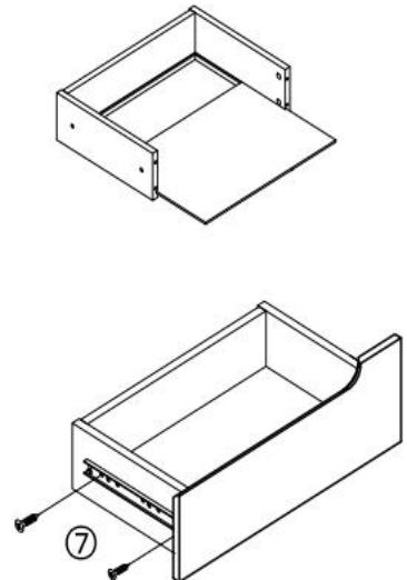
10、The 18 adopts ① and ② to connect the 19, then insert 20. The 18 adopts ① and ② to connect the 16, then use ⑦Install the ⑪ on the outside of the 18.
