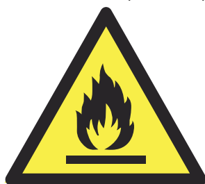
Caution: Risk of fire/ flammable materials
