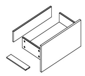
4. Use ③,④,⑤ to connect and fix the 7, 8, 9, and insert the 11, and then lock the 10. Install the ⑩-B at the reserved hole on the outside of the d9 using ②, put the drawer into the cabinet.
