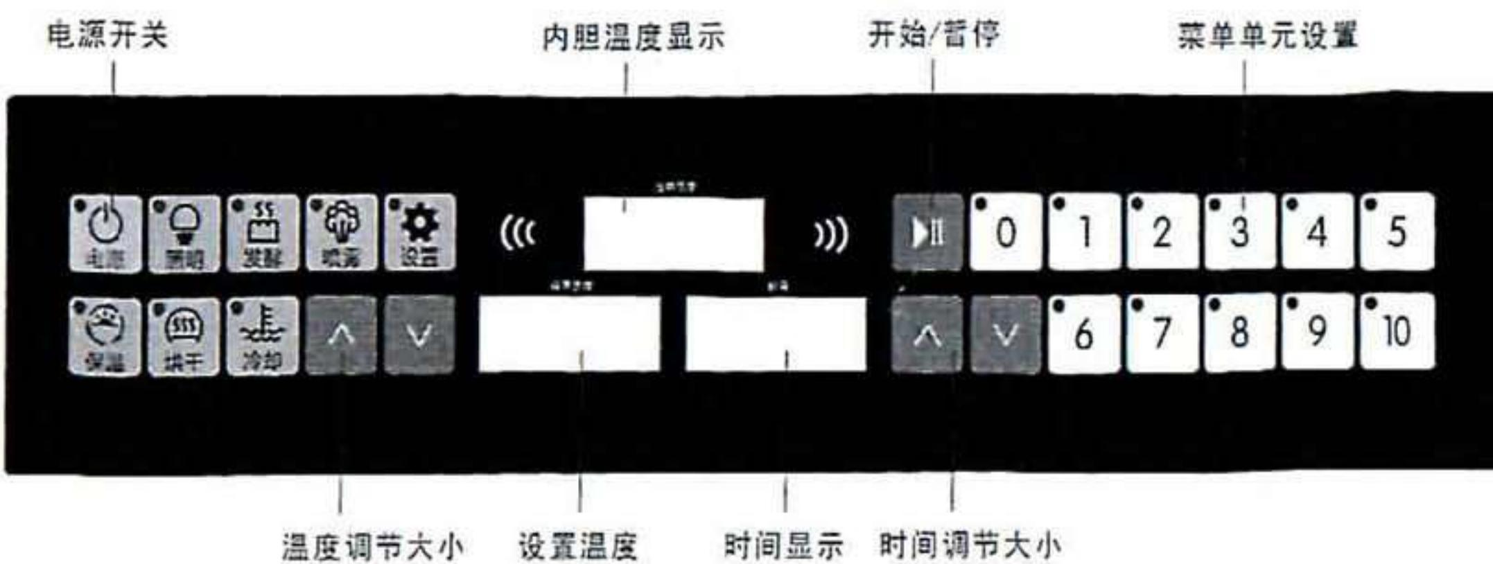
**Power switch:** long press 2s to turn on or turn off the power; short press once to reset (when you need to use other function, you can short press the power button, then choose the function you need).
