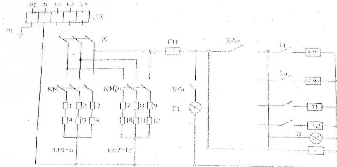
**KM1:** Upper heating element alternating current contactor
